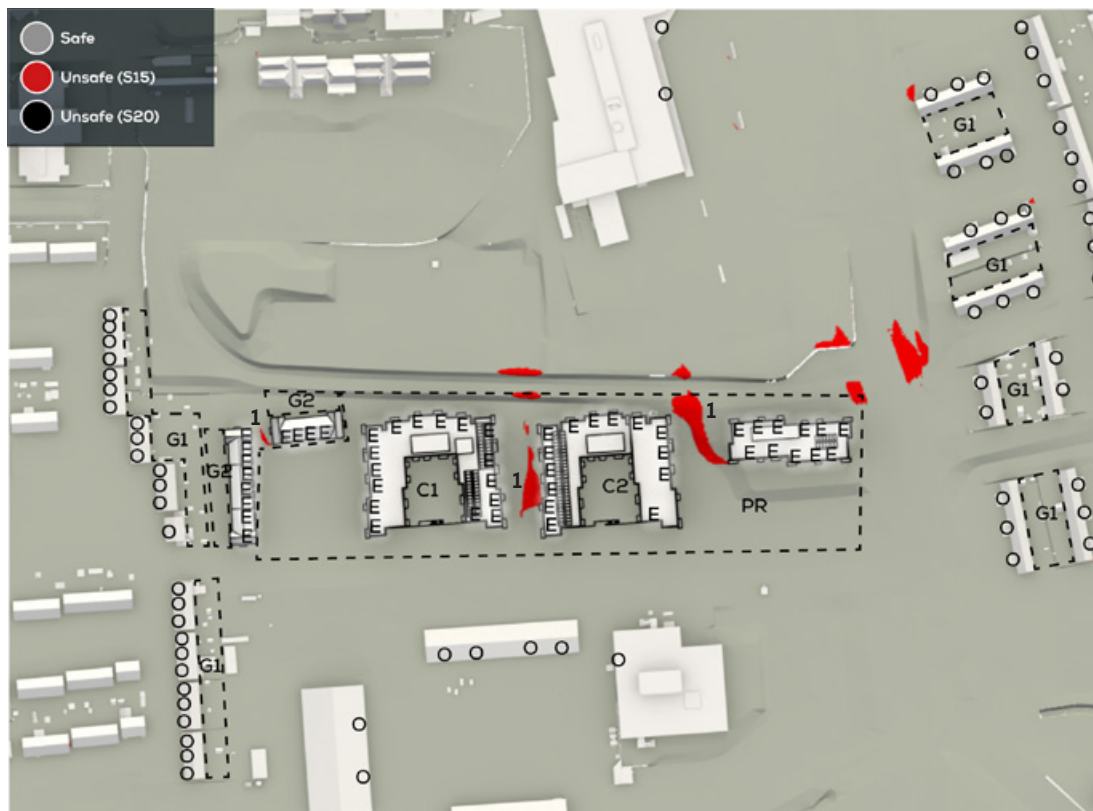
Fig. 08: Annual Safety at Ground Level, Section 32B Scheme with Existing Surrounds
