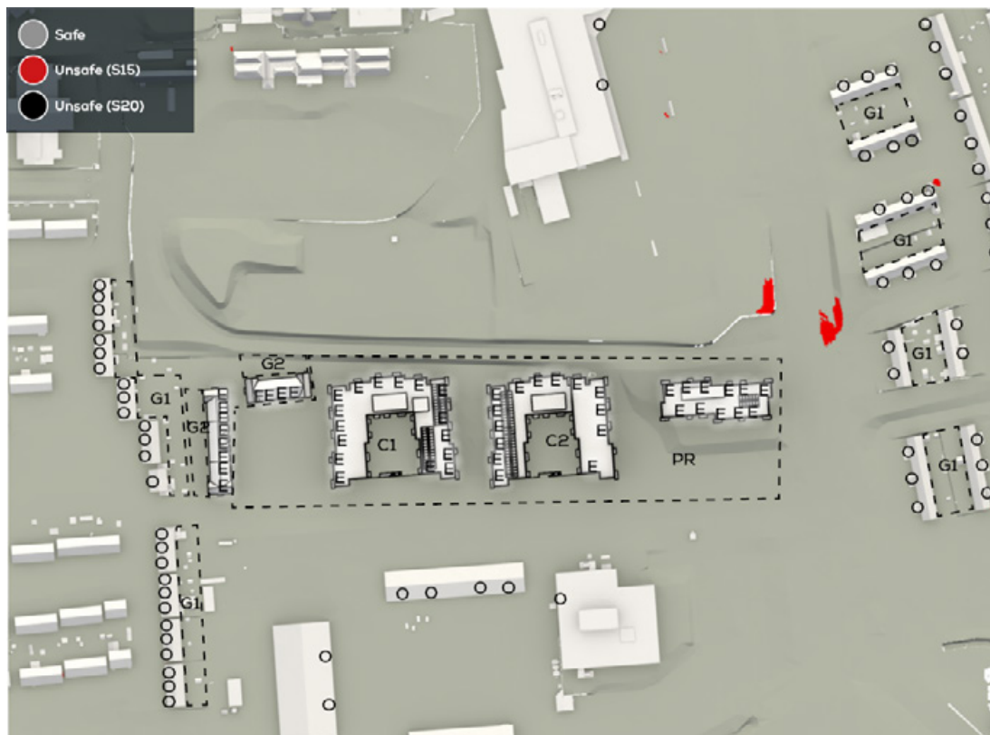
Fig. 22: Annual Safety at Ground Level, Section 32B Scheme with Landscaping, Mitigation and Existing Surrounds
