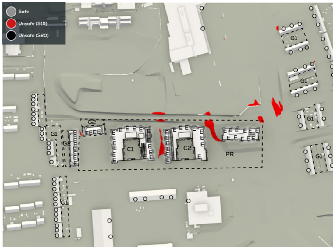
Fig. 14: Annual Safety at Ground Level, Section 32B Scheme with Cumulative Surrounds
